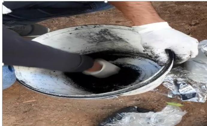
Figure 15: Mixing of rubber particles with PU glue
