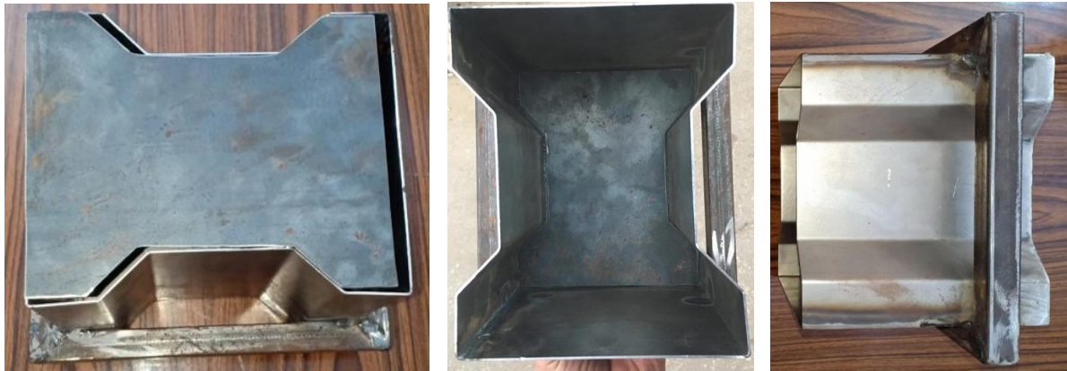
Fig 20: Initial sheet metal mold
