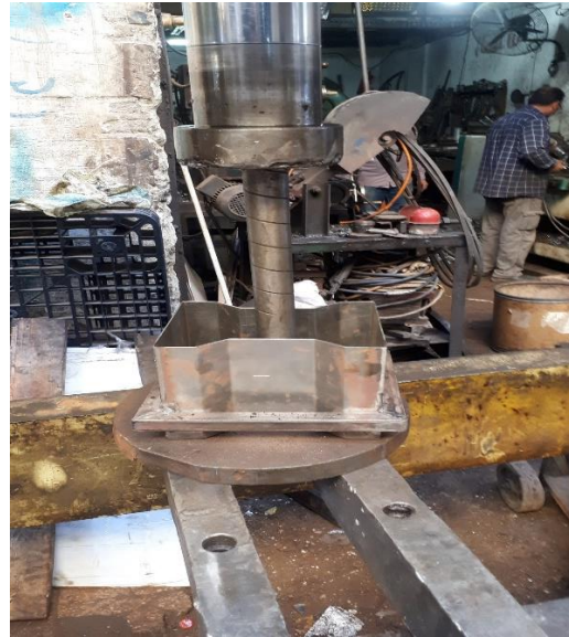
Figure 16: Pressing of rubber mixture with force of 8 ton
