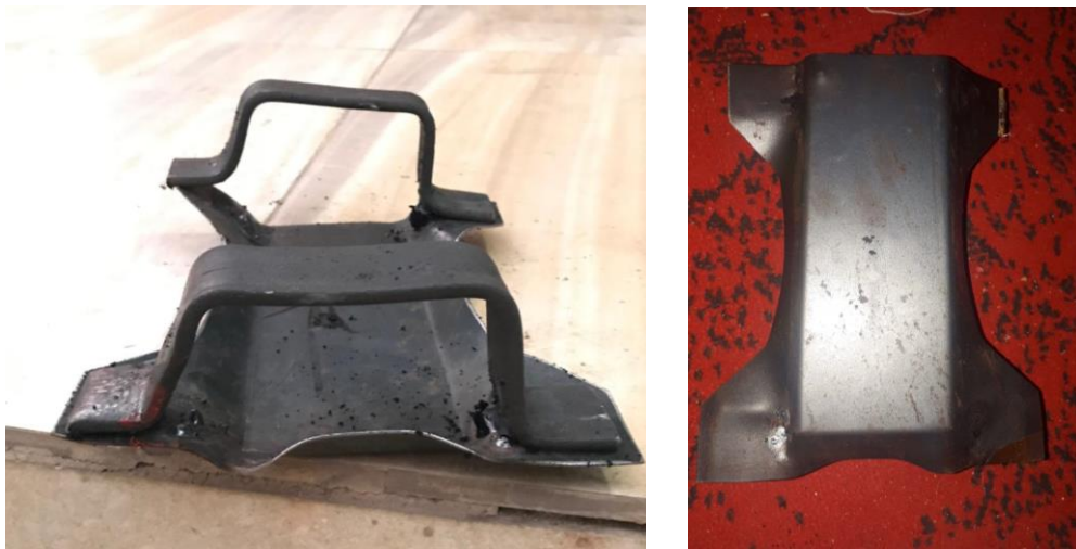
Fig 21: Initial mold male failure
