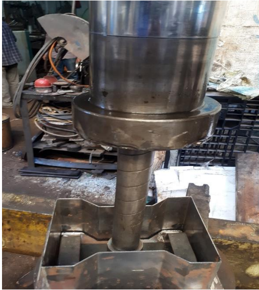
Figure 16: Pressing of rubber mixture with force of 8 ton
